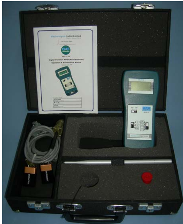
Figure 2 Standard package for IRD811D Digital Vibration/Spike Energy Detector
