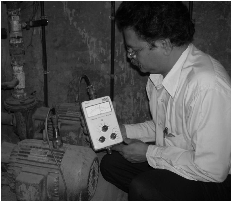
Figure 1 Periodic Vibration measurements save valuable machine downtime
