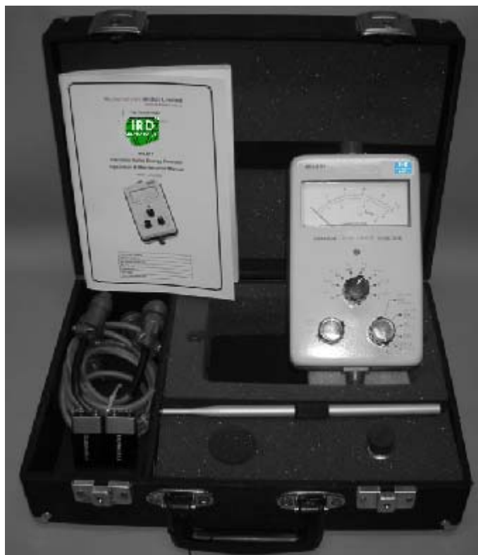
Figure 2 Standard package for IRD 811 Vibration-SPIKE ENERGY Detector
