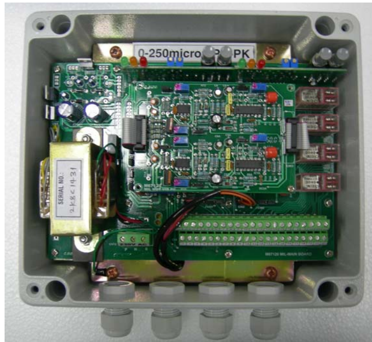
Figure 3 Blown out view of the machinery protection transmitter dual-channel (IRD 7120)
