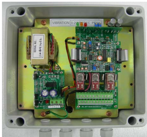
Figure 2 Blown out view of Machinery protection transmitter 1-ch IRD 7110
