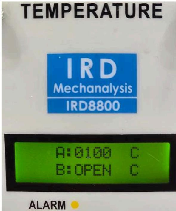
Our Online Systems IRD7100 MPT as well as IRD8800 MPS API670 also come for Temperature Measurement. The sensor used is either a PT100 RTD or a Dual Output Vibration cum Temperature Sensor (like IRD515). Contact Surface Temperature can be measured in both Degrees Celsius as well as Degrees Fahrenheit. 4-20 mA output, MODBUS Output, Relay Contacts and more are available to Monitoring and Protection. The Data can also be integrated to our Cloud Based Systems as well as OLIVER™
