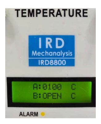
Our Online Systems IRD7100 MPT as well as IRD8800 MPS API670 also come for Temperature Measurement. The sensor used is either a PT100 RTD or a Dual Output Vibration cum Temperature Sensor (like IRD515). Contact Surface Temperature can be measured in both Degrees Celsius as well as Degrees Fahrenheit. 4-20 mA output, MODBUS Output, Relay Contacts and more are available to Monitoring and Protection. The Data can also be integrated to our Cloud Based Systems as well as OLIVER<sup>™</sup>
