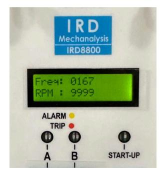
Our Online Systems IRD7100 MPT as well as IRD8800 MPS API670 also come for Speed Measurement. We utilise either Laser Based Tachometers or Eddy Current Based Non-Contact Sensors for Speed Measurement. Laser Based Tachometers require a Reflective Tape or Reflective Patch on rotating shaft for Speed detection. Eddy Current Based Non-Contact Sensors need a Notch or a Toothed Wheel on the Rotating Shaft for Speed measurement.
